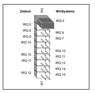
Figure 2-6 shows the setting for IRQ5 in a WinSystems AT-compatible computer.
